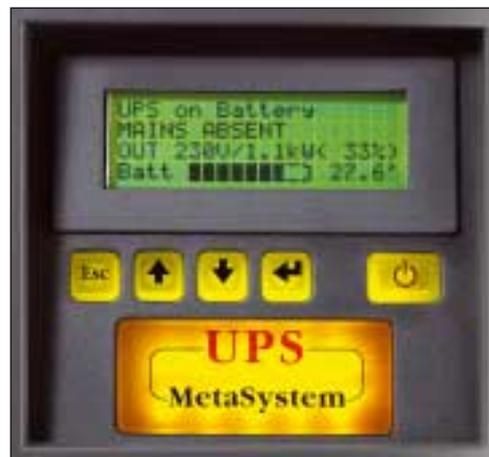
More expert users have the option of setting the mode for the exploitation of the backup energy based on battery voltage thresholds, predetermined operating time limits or according to the Status Of Charge of the batteries.
